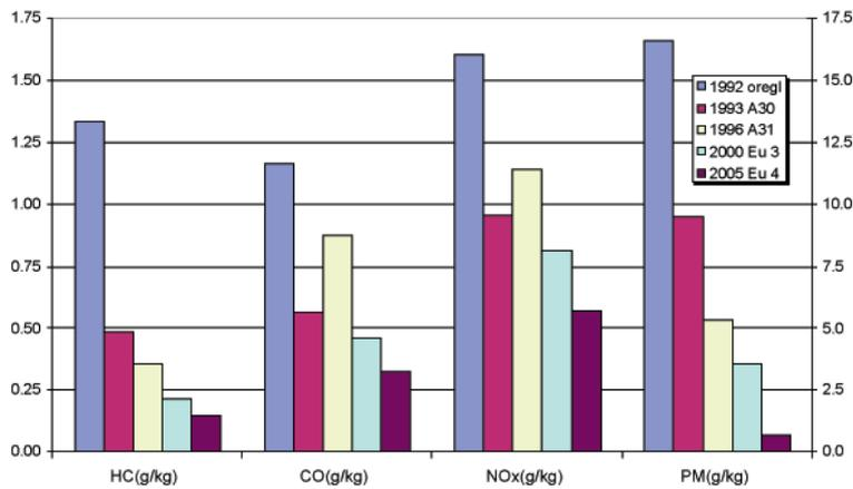
Figure 2. Emissions for diesel-powered buses without aftertreatment
