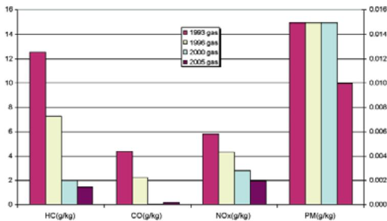
Figure 3. Emissions for gas-powered buses with catalytic converters
